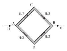
Heat current will flow from A to B via path ACB and ADB. Since all the rod are identical, so,  $(\Delta\theta)_{AC} = (\Delta\theta)_{AD}$
