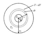
To measure the radial rate of heat flow, integration technique is used, since the area of the surface through which heat will flow is not constant.
